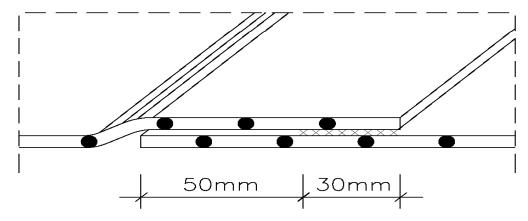
Lap joint without air-channel (single weld)
