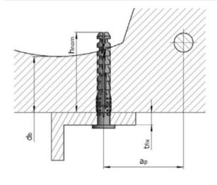
$h_{\mathsf{nom}}$ = overall plastic anchor embedment depth in the base material
