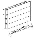
ISO SPAN - shuttering blocks made of wood-chip concrete
