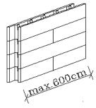
THERMOSPAN - shuttering blocks made of wood-chip concrete
