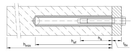
$t_{fix}$  = thickness of fixture
