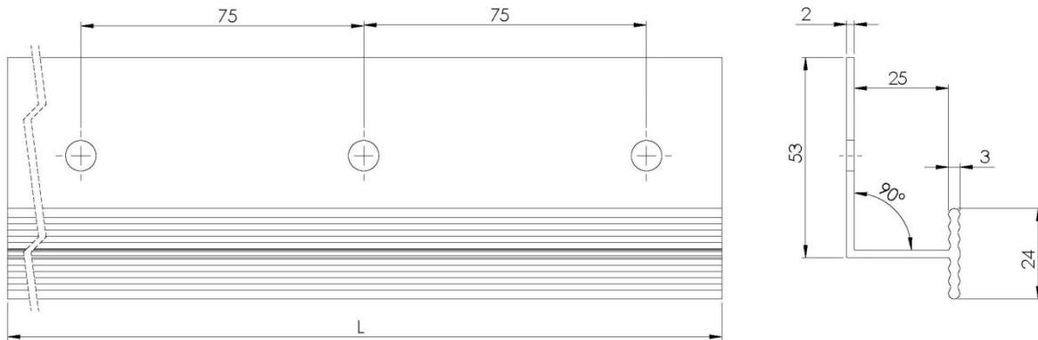
**Vertical connection profile – "Verbindungsleiste PVC"** (dimensions in millimetres)
