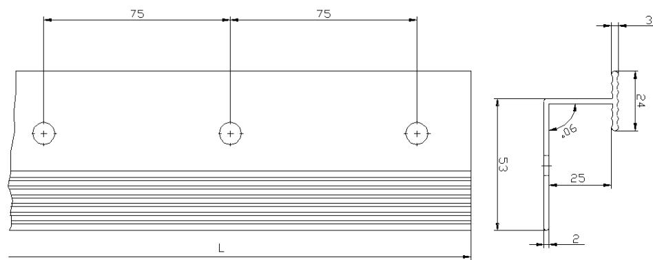
**Vertical connection profile "Brillux WDVS Verbindungsleiste 3544"** (dimensions in millimetres)
