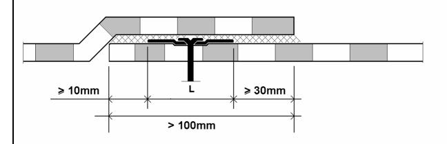
Overlap design for DUO application (self adhesive part + torched part). This is the SOPRAFIX STICK case.
