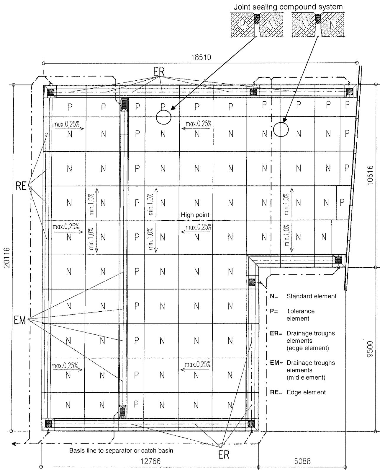
BTE Stelcon pre-fabricated elements of reinforced concrete
