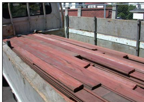
Figure 3 Jarrah flooring recovered for reuse from St Joseph's Church in Wellington
