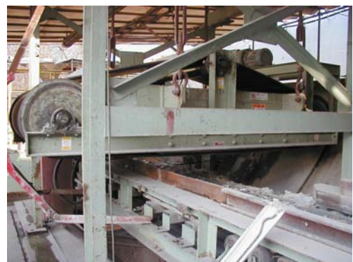
Photo 6 Metal removal by magnetic separator
