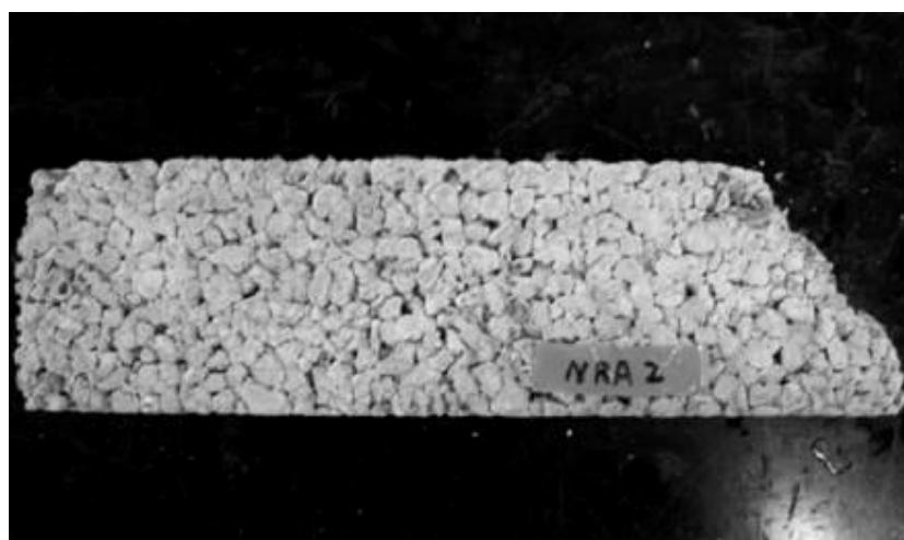
Figure 4. Typical fracture patterns after ASTM C666 test procedure B (NR6).
