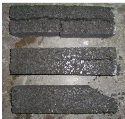
Figure 2. Typical fracture patterns after ASTM C666 test procedure A (NR6).
