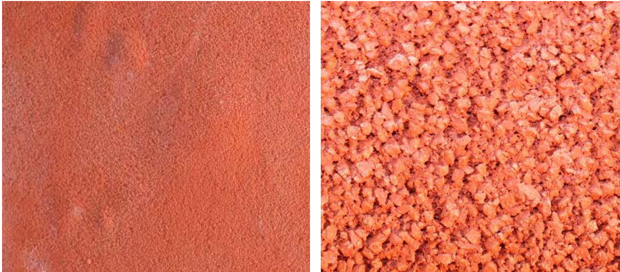
Figure 6. (Left side) Photograph of ETICS finish coat at ageing time T1; blisters (larger ones: 10 cm diameter circa) are evident on the surface of the sample; (Right-side) dimension of pores and surface appearance are changed (aggregate dimension 0/1 mm); Localized fading due to rain-wash is shown.
