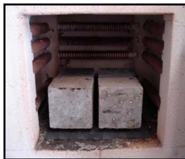
Figure 1. Specimens in the electrical furnace
