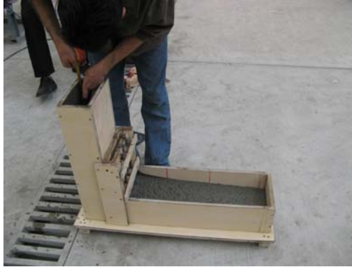
Figure 6. Schematic illustration of L-box
