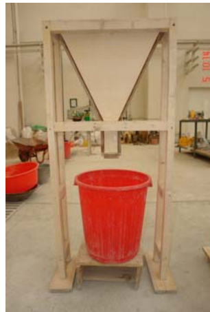
Figure 5. Schematic illustration of V-funnel
