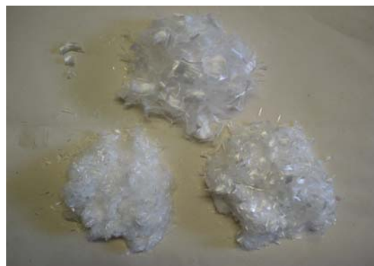
Figure 3. Sample of polypropylene fibers (6, 12 and 19 mm)
