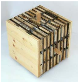
Figure 1 The prototype Timber Block “Klimablokka” made of reclaimed wood. [1]
