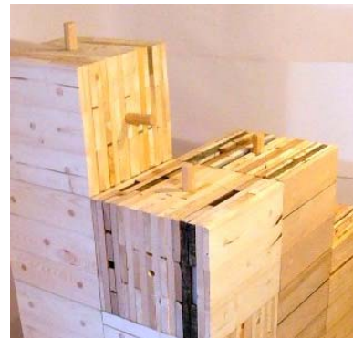
Figure 4 The prototype Timber Block as a stacked construction system using plugs. [1]
