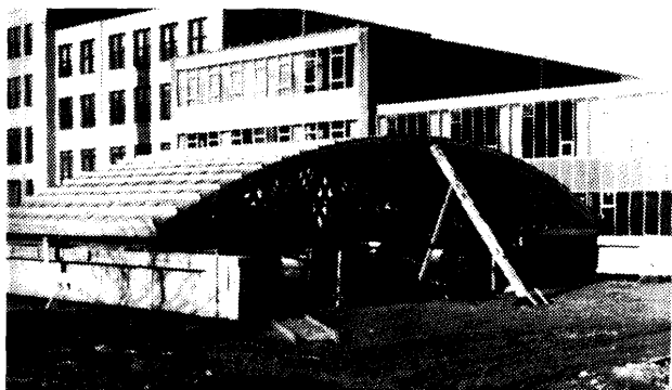
Figure 3. Set-up for test on roof trusses of 60 ft. span.
