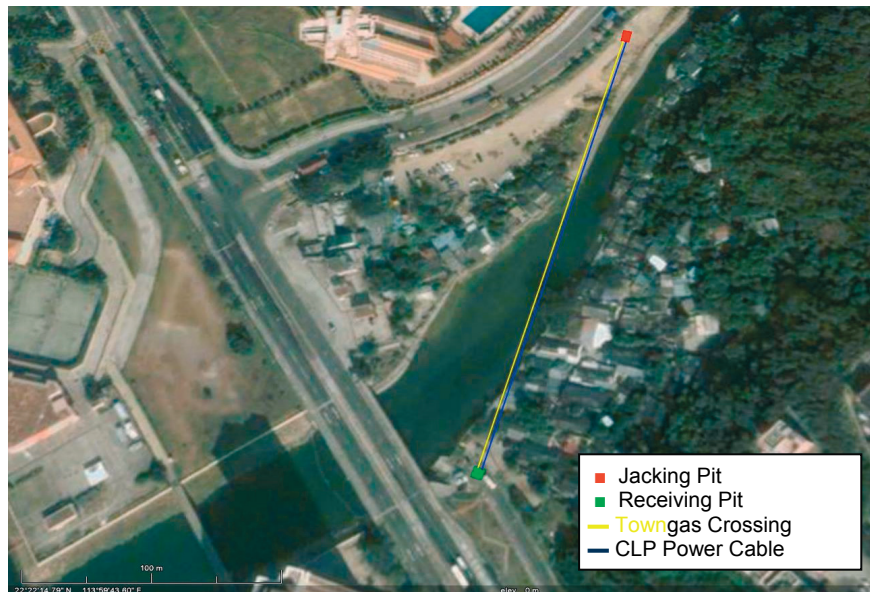
Fig. 3 – Site overview of case study microtunneling project
