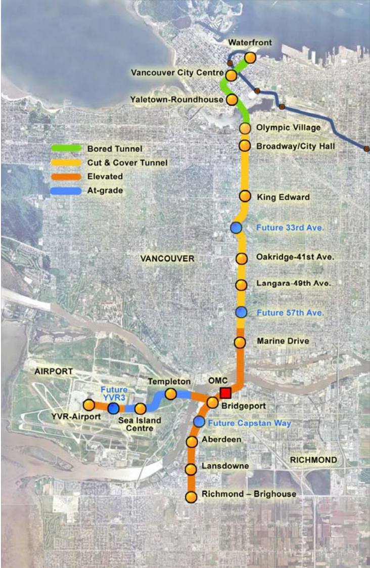
Figure 1. Canada Line alignment
