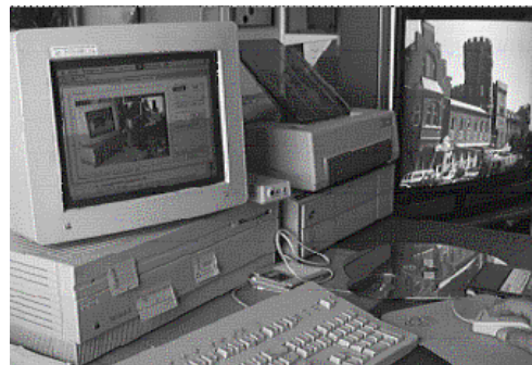
Figure 1: Left; Experimental set-up at KBS-Media Lab, Lund University, 1991, with video communication and screen sharing using Timbuktu from Farallon. Right; A hypermedia workstation developed 1988 at KBS-Media Lab, Lund University with video display of images and films stored on video disk integrated with the hypertext based program HyperCard from Apple computer. From (Christiansson 2001b).
