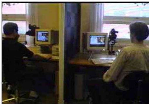
Figure 1: Left; Experimental set-up at KBS-Media Lab, Lund University, 1991, with video communication and screen sharing using Timbuktu from Farallon. Right; A hypermedia workstation developed 1988 at KBS-Media Lab, Lund University with video display of images and films stored on video disk integrated with the hypertext based program HyperCard from Apple computer. From (Christiansson 2001b).
