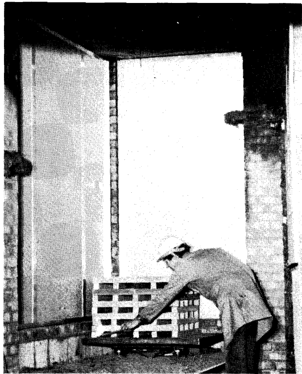
Figure 1 Corner-wall test rig showing panels and crib before test
