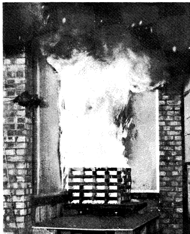
Figure 2 Corner-wall fire test in progress
