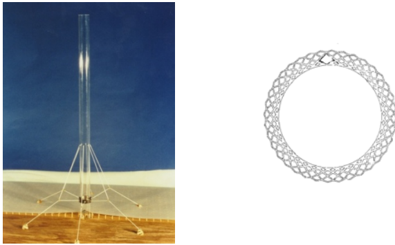
Figure 6. Model of a 600 meter high solar chimney and its cross-sectional plan representing a porous organic form (source: the authors)
