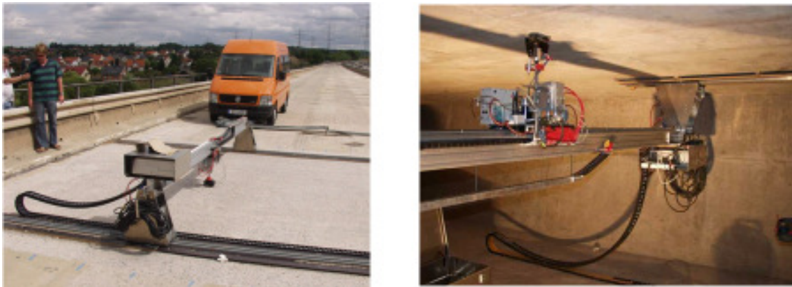
FIGURE 6. Ultrasonic-scanner for application on bridge decks and inside a box girder.
