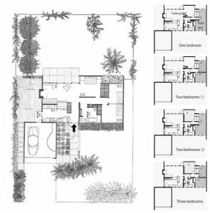
Figure 9: Typical plan and four types of room configurations
