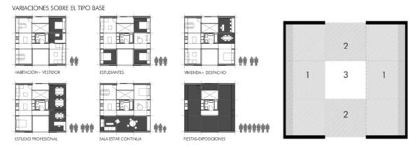
Figure 10: Flexible layout typology & different areas: 1-living, 2-bioclimatic, 3-services
