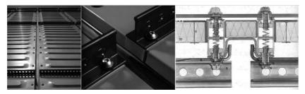
fig.16: panel jointing, images and horizontal section detail.
