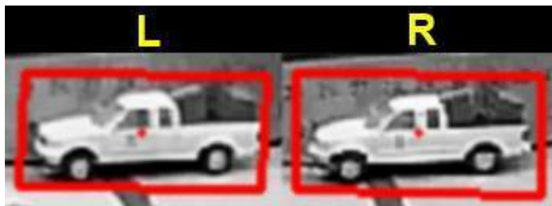
Fig 5: Differing centroid position P_L and P_R after 2D tracking in video frame #127
