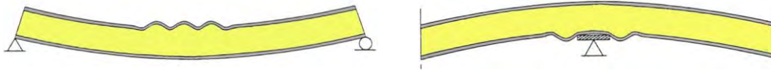
Figure 2. a) Wrinkling failure in a span and b) on an intermediate support.
