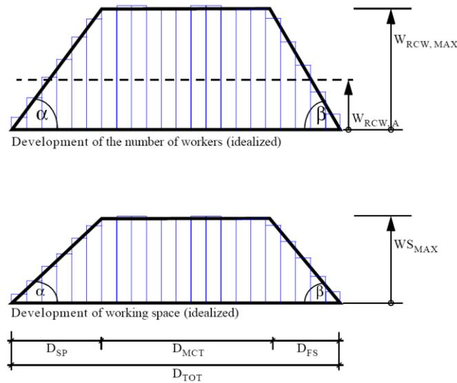
Figure 2: Correlation between number of workers and available workspace for reinforced concrete works
