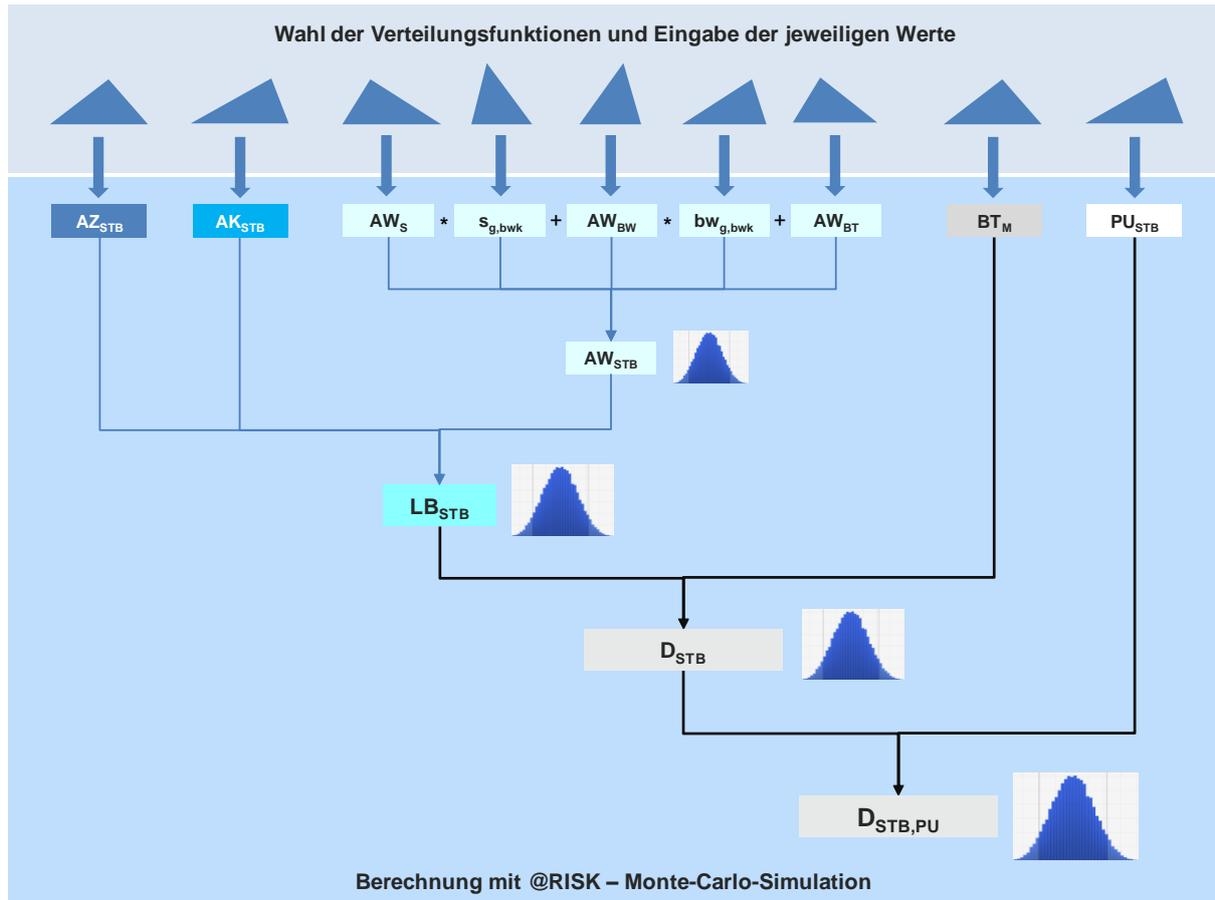
Figure 3: Calculation Mode 3 – construction time: Flow chart
