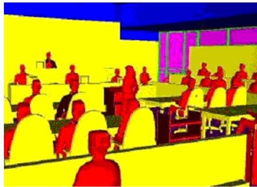
Figure 8. Conversion of format led to loss of colors and textures from the 3D CAD model.
