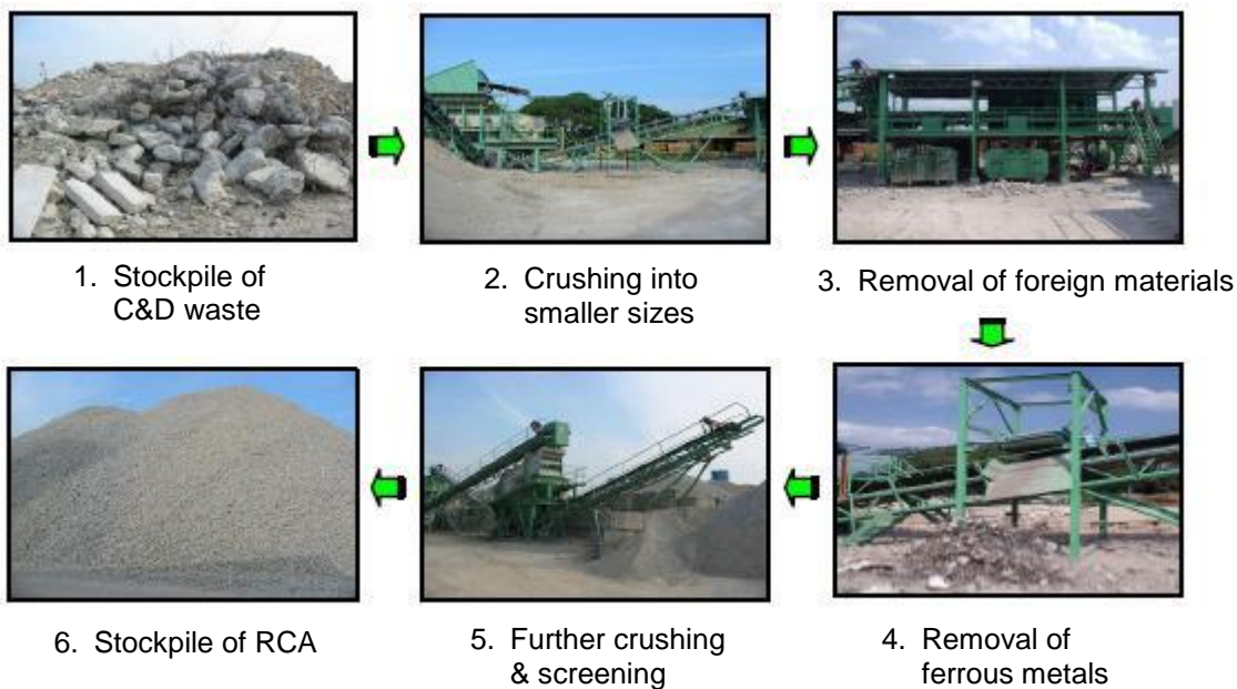
Figure 3: Processing of C&D Waste into RCA
