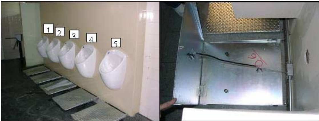
Figure 4 – Measurement system - platforms with sensors
