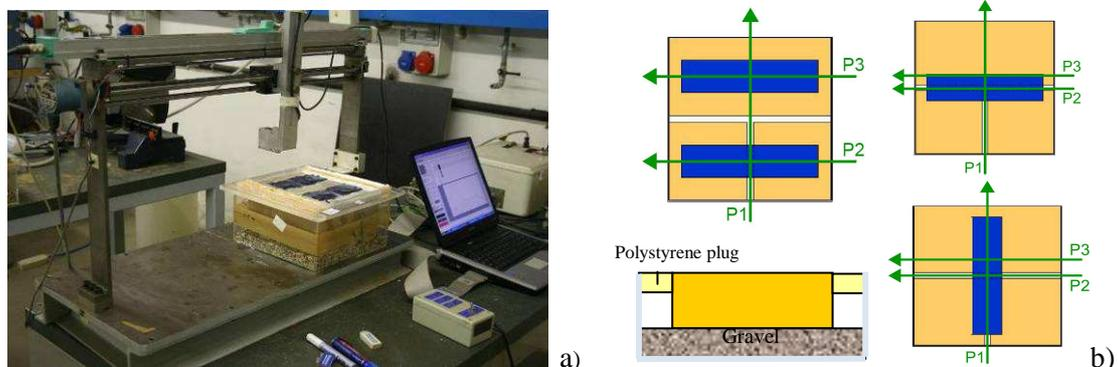
**Figure 4.** Damage measuring device: a) lasers profilometer, b) scheme of the measurement.
