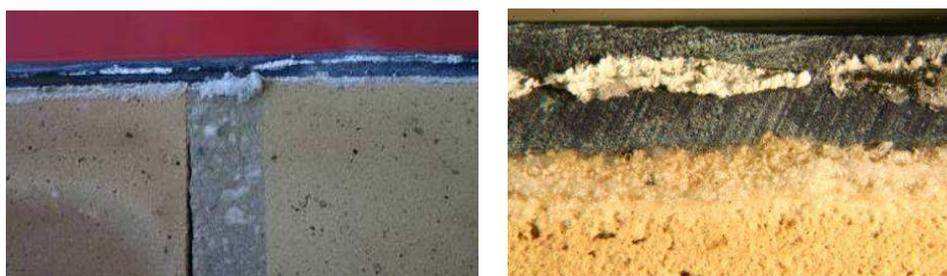
**Figure 10.** A vertical section of the specimen upper surfaces. Subefflorescence at the depth of penetration of the primal into the brick and within the FRP strip
