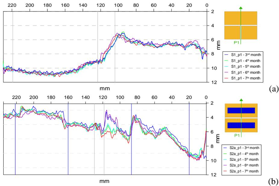
**Figure 6.** Diagrams of the profiles for specimens S1 (a), and S2a (b) measured at cycles 3, 4, 5, 6 and 7
