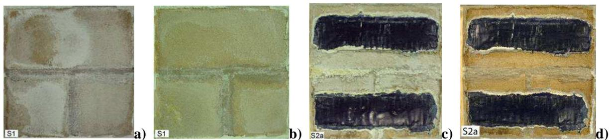
**Figure 5.** a), b) blank specimen S1 before and after brushing; c), d) specimen S2a before and after brushing.
