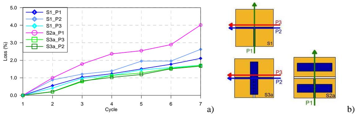
**Figure 7.** a) Area loss % against number of cycles for some of the obtained profiles, b) specimens and profiles.
