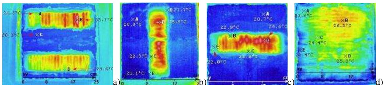
**Figure 9.** Thermographic restitution of S2a, S3a, S4a, S5a upper face after 7 cycles
