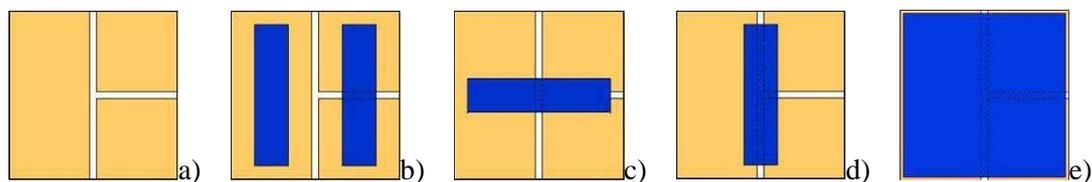
**Figure 1.** Soldier course specimens for crystallisation tests: a) S1; S1a, plain sample (only brickwork); b) S2, S2a, configuration 1, c) S3, S3a; configuration 2, d) S4, S4a; configuration 3, 4) S5, S5a, configuration 4, FRP covering the whole surface of the specimen.
