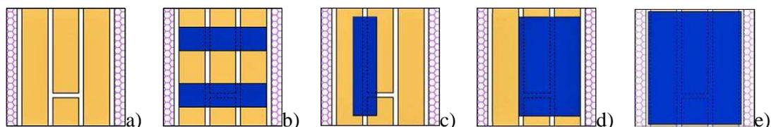
**Figure 2.** Running bond specimens for crystallisation tests: a) T1; T1a, plain sample, (only brickwork); b) T2, T2a, configuration 1, c) T3, T3a; configuration 2, d) T4, T4a; configuration 3, 4) T5, T5a, configuration 4, FRP covering the whole surface of the specimen.
