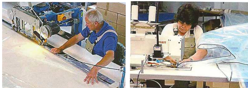
Figure 1 and 2. Jointing of ETFE-foils by hot fusion and inlay of keder in foil boundary loop.
