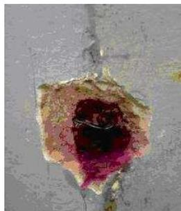
**Figure 5.** The color shows the carbonation of concrete in column P2.
