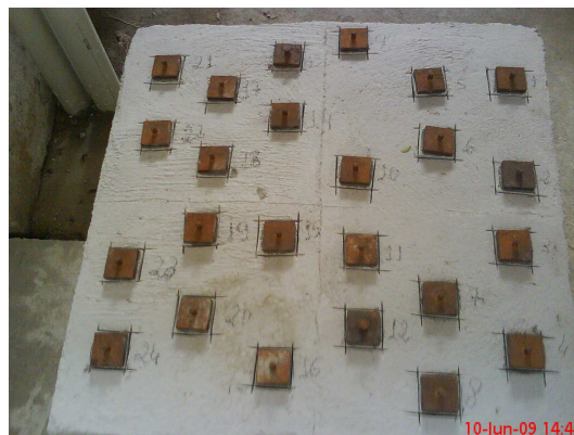
Figure 6. Samples prepared for the test to determine adhesion strength.
