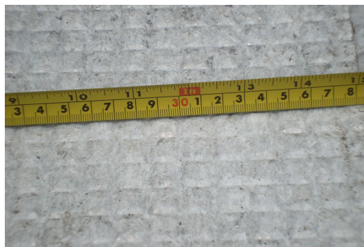
Figure 3. Geometric detail of the textured mold with closed grooves.
