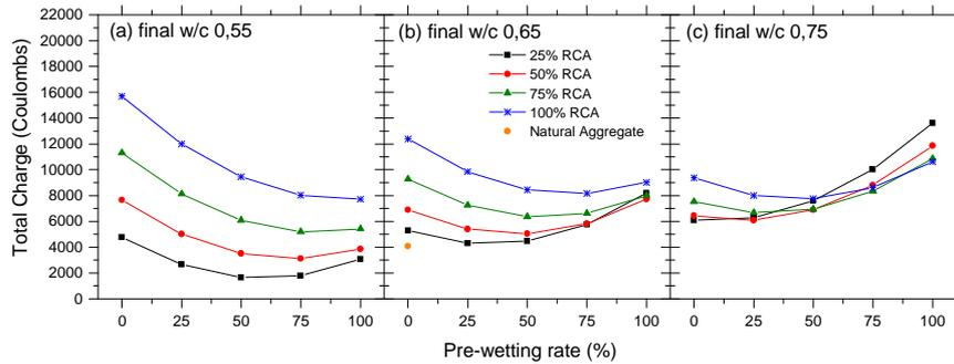
**Figure 3.** Total charge for concrete with RCA 37 MPa.
