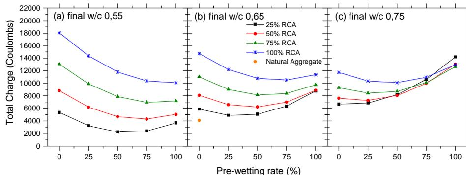
**Figure 2.** Total charge for concrete with RCA 18 MPa.
