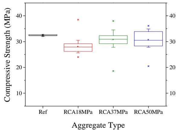
**Figure 1.** Effect of compressive strength of RCA on compressive strength of new concrete.
