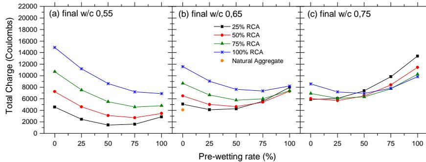
**Figure 4.** Total charge for concrete with RCA 50 MPa.
