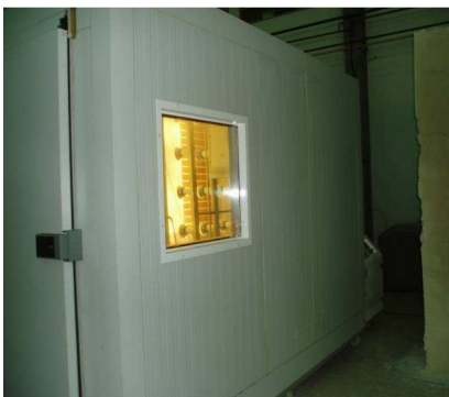
Figure 1. ETICS subjected to hygrothermal cyclic testing (with 80 mm and with 1 to 2 mm joint widths).
