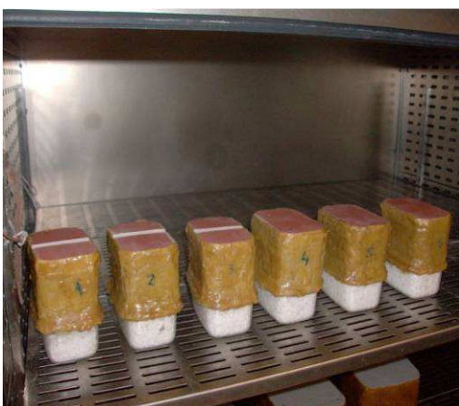
Figure 5. Test of water vapour permeability.
