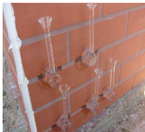
Figure 6. Water permeability under low pressure test with Karsten tubes.
