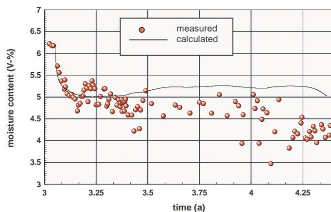
Fig. 8. Measured and calculated wood moisture content 12 cm from the beam head with heating pipe, Jan. 19,1998 to May 5, 1999
