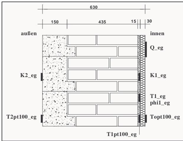
Fig. 2. Wall construction and sensor location in the ground floor of the test building in Dresden
