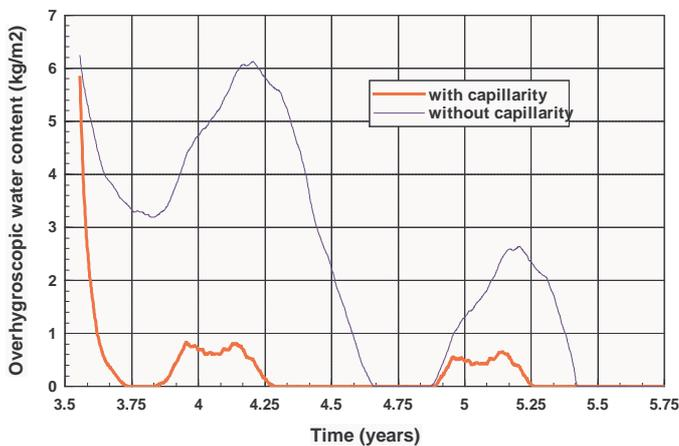
Fig. 16. Test building in East Saxony: comparison of the integral overhygroscopic water mass in the construction with and without consideration of capillarity
