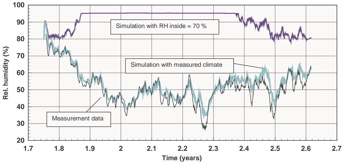
Fig. 10. Herrenschiesshaus Nuremberg: Measurement data and simulation of the relative humidity between insulation and original wall, starting from the application of the insulation boards
