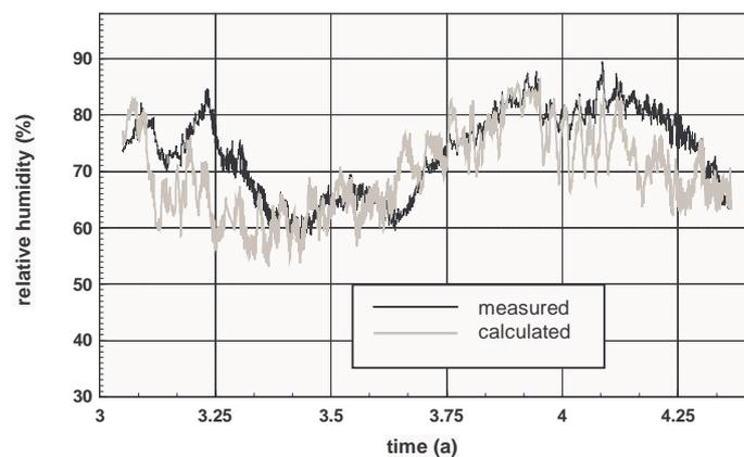
Fig. 7. Measured and calculated relative humidity in the air space at the beam head with heating pipe, Jan. 19,1998 to May 5, 1999
