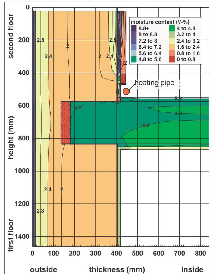
Fig. 6. Senftenberg: Moisture field around the wooden beam head with calcium silicate inside insulation and heating pipe
