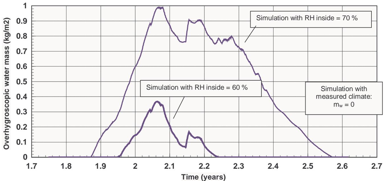
Fig. 11. Herrenschiesshaus Nuremberg: Overhygroscopic water mass in the construction for several indoor air humidities
