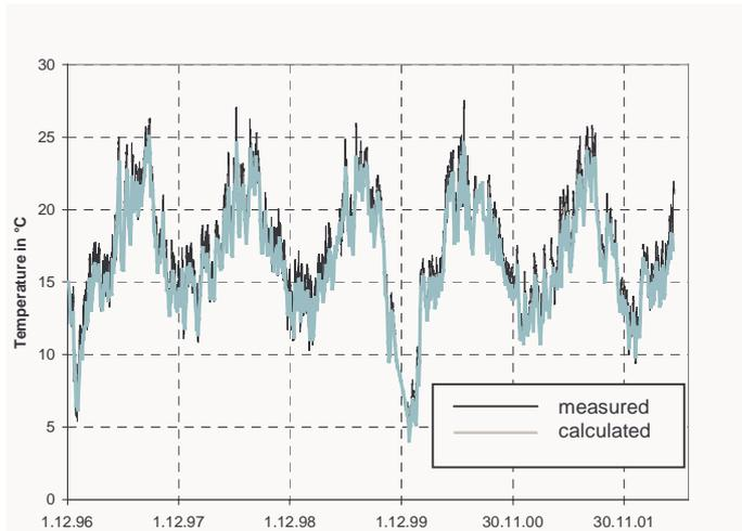
Fig. 3 Measured and calculated temperature between old inside plaster and coupling mortar, time from Dec. 5, 1996 to June 11, 2001
