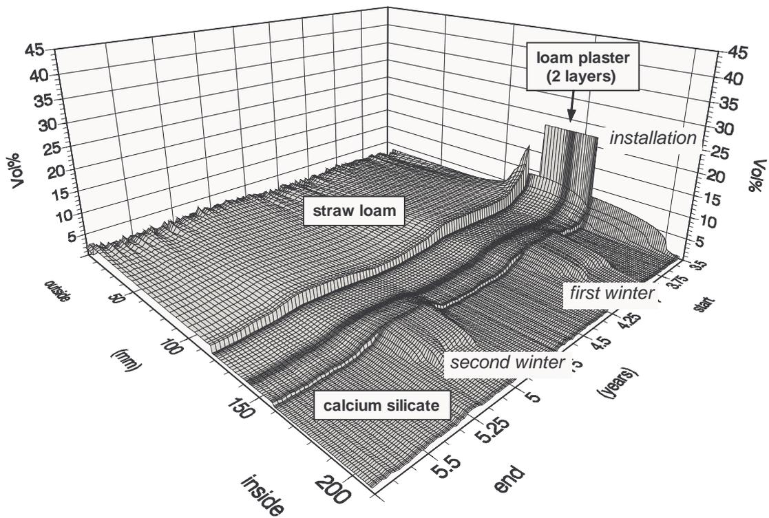
Fig. 14: Water content profile in the center of the straw loam field (one-dimensional simulation) with measured capillary conductivity for all materials
