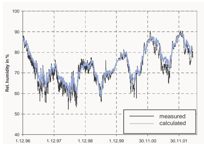
Fig. 4: Measured and calculated relative humidity between old inside plaster and coupling mortar, time from Dec. 5, 1996 to June 11, 2001
