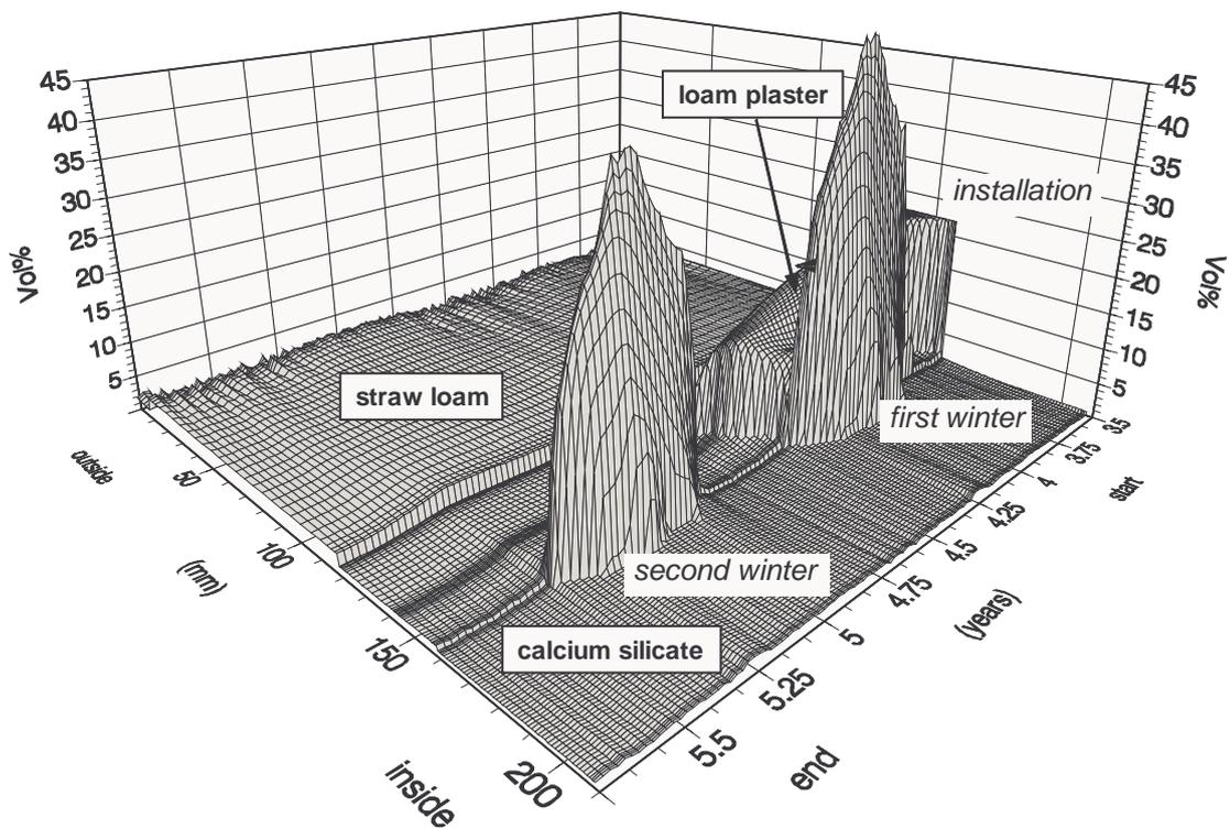
Fig. 15: Water content profile in the center of the straw loam in time (one-dimensional simulation) without consideration of capillary forces of all materials
