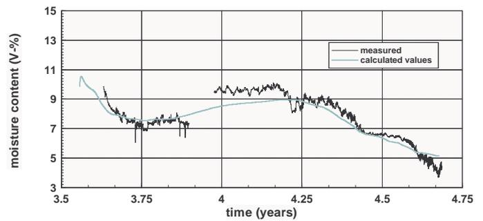
Fig. 13. Measured and calculated moisture content in 13mm depth in the wooden beam (calcium silicate insulation with straw loam filling)
