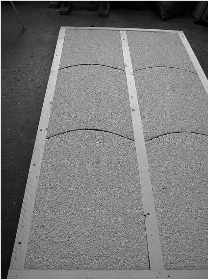
Figure 3. Opened wall with wood shavings after tests.
