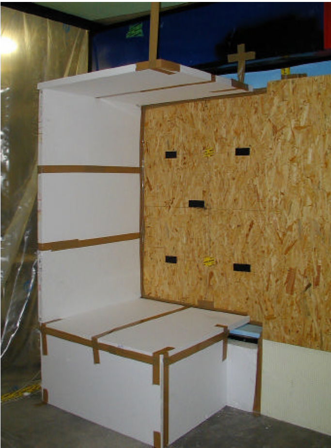
Figure 4: Top: 3 wall elements in double climate chamber (seen from warm side). Bottom: simulated corner (ceiling, wall, floor).
