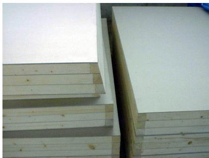
Figure 4: Panels showing timber edge
