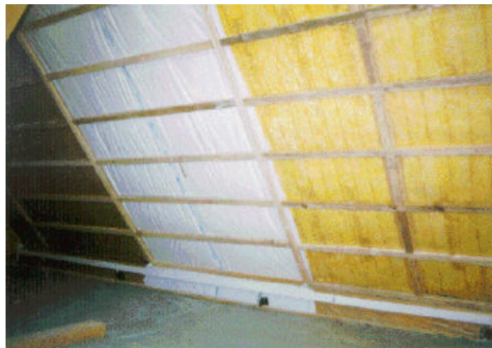
Figure 7. The tested roof covered with metal sheets. Top: Basic design of the test sections. Bottom: Photographical view of the interior.
