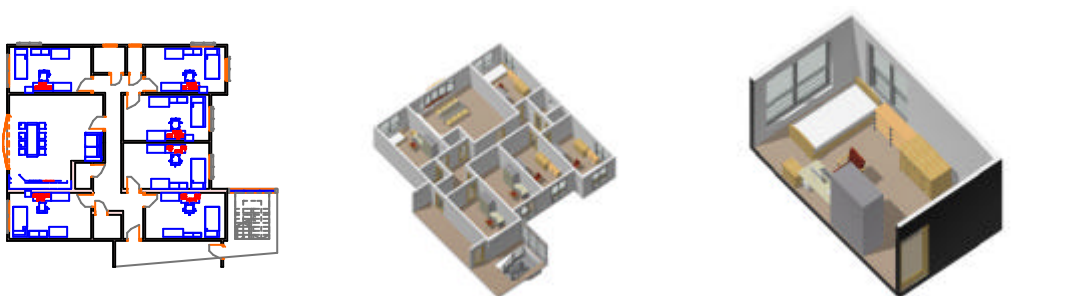
Figure 4. Conventional (left hand view) and object oriented modes (centre and right hand views) of representing the same area from a case study student project under design
