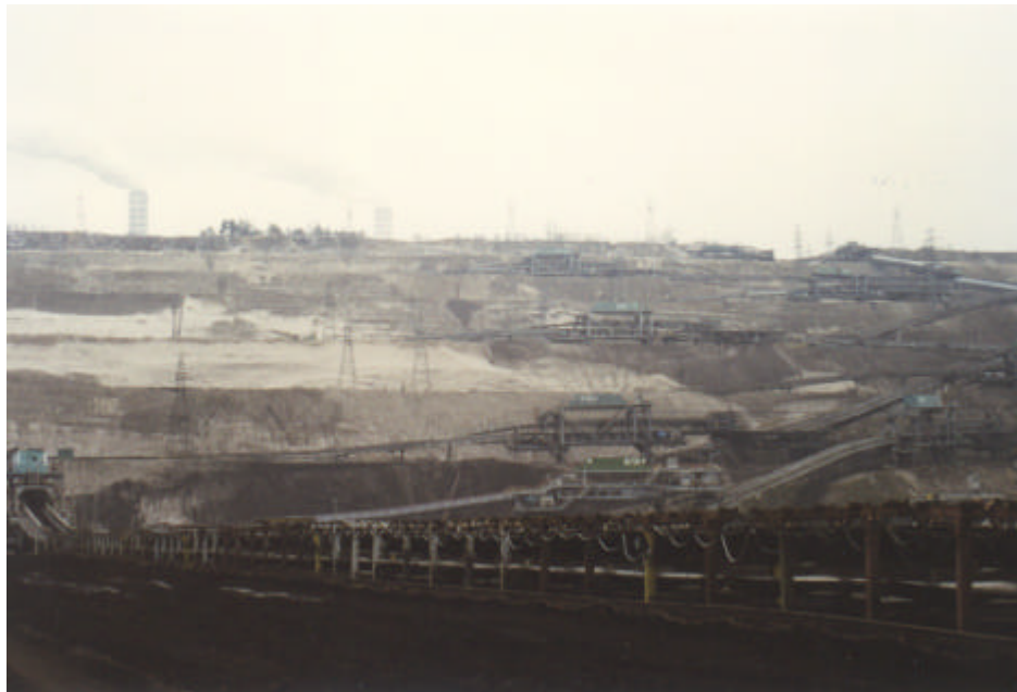
Fig. 4 Open pit of lignite mine Belchatów. Length of lignite deposit-30 km, width 1,6 km. Depth of the pit 300 m. Power plant gives 25 % of polish requirements for electrical energy.
