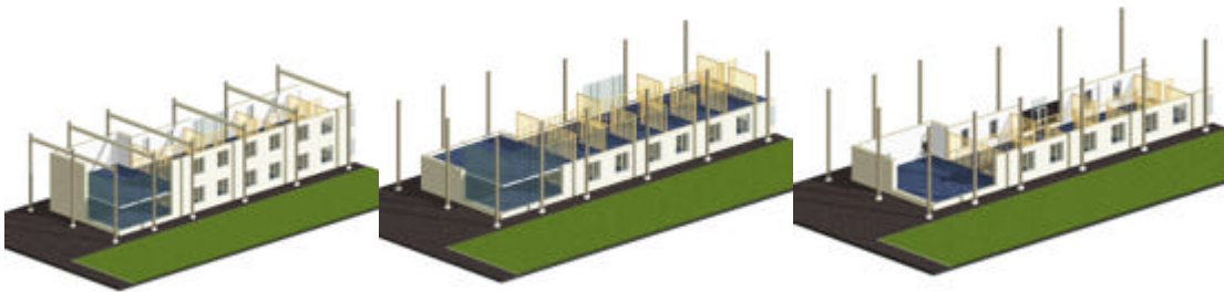
Figure 6. Sequential views from a building information model of a student project showing the progressive sequence of disassembly at the end of service life following Catalli's [30] principles
