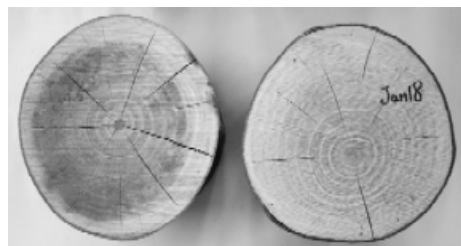
Figure 3 The cut surface of Japanese dogwood felled at waning moon phase (right) and at waxing moon phase(left) aged with branches
