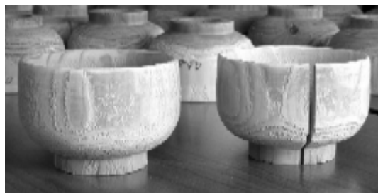
Figure 1 Intact bowl made from wood felled at waning moon phase aged with branches (forward, left) and cracked bowl made from wood felled at waxing moon phase aged without branches (forward, right)
