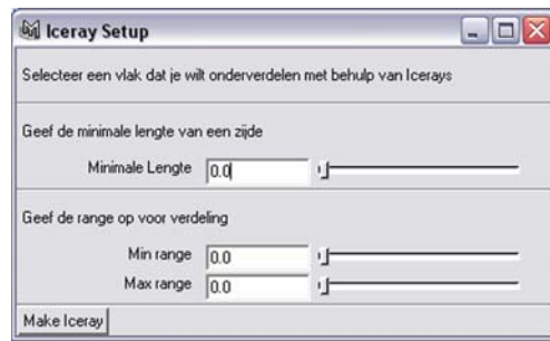
Figure 5. The user interface to specify the minimal length constraint (“Minimale Lengte”) and the parameter values (“Min range” and “Max range”) that serve to define the section of the polygon's edge wherein the endpoint of the single line (rules 1 through 4) lies.
