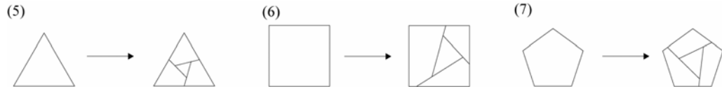
Figure 3. Three additional constructive rules that inscribe a triangular shape between three edges of a triangle, convex quadrilateral or pentagon.
