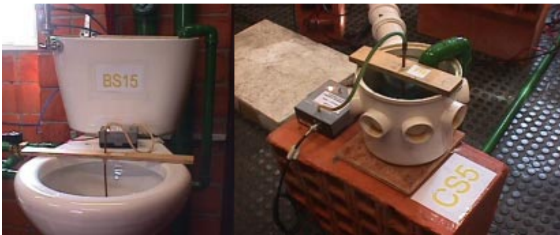
Water closet trap seal
