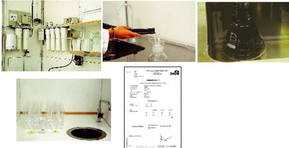
Figure 13 - Steps of taste and odour control of the raw material and pipe
