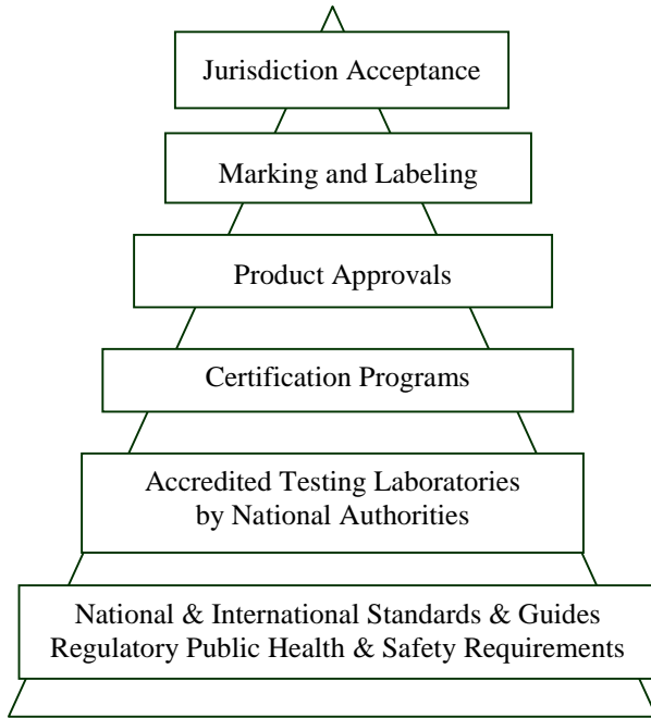
LADDER for NECESSARY PROCEDURES
