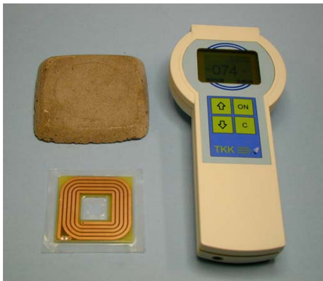
Fig. 1. Pre-cast basic sensor, basic sensor and reading device
