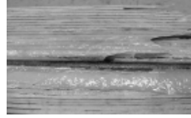
Figure 8. De-bonding between adhesive and steel leading to interfacial slip.
