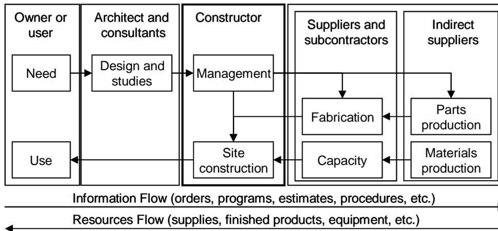
Fig. 2 General model of the supply chain in construction (adapted from Vrijhoef y Koskela, 1999)
