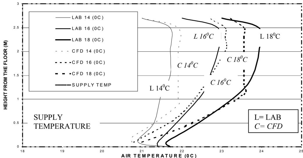
**Figure 5.** Air temperature versus height above the floor for a range of ceiling temperatures, and at fixed heat load of 40W/m<sup>2</sup> and 3.9 ACH.
