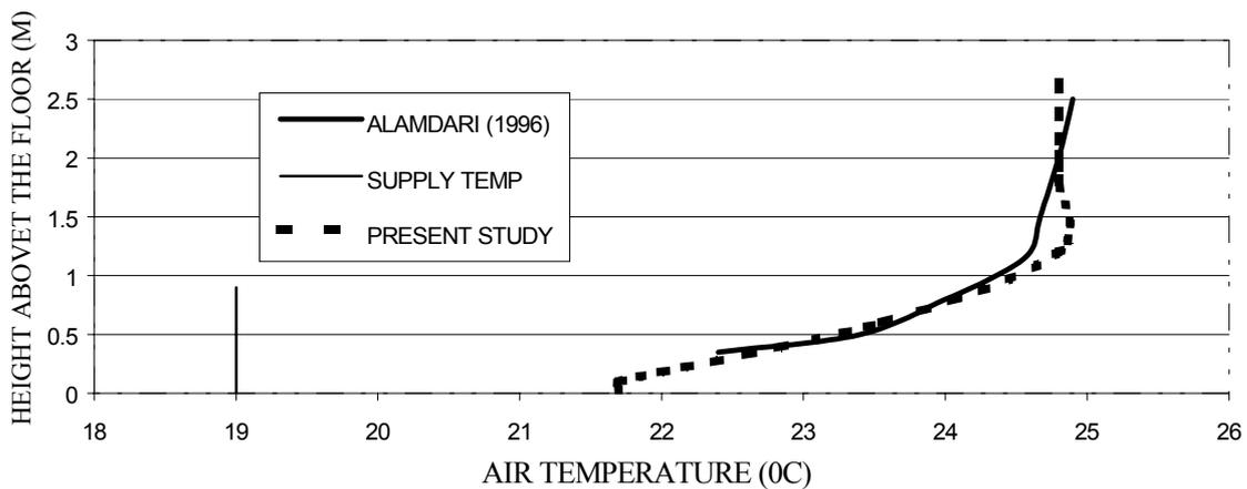
**Figure 4.** Air temperature versus height above the floor, for ceiling temperature 16°C, 3.5ACH and 60W/m<sup>2</sup>: comparison of this with (Alamdari and Eagles, 1997)
