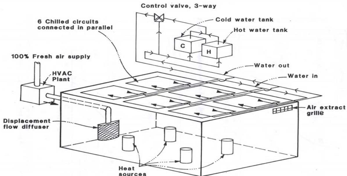
**Figure 1.** Schematic diagram of the room being modelled
