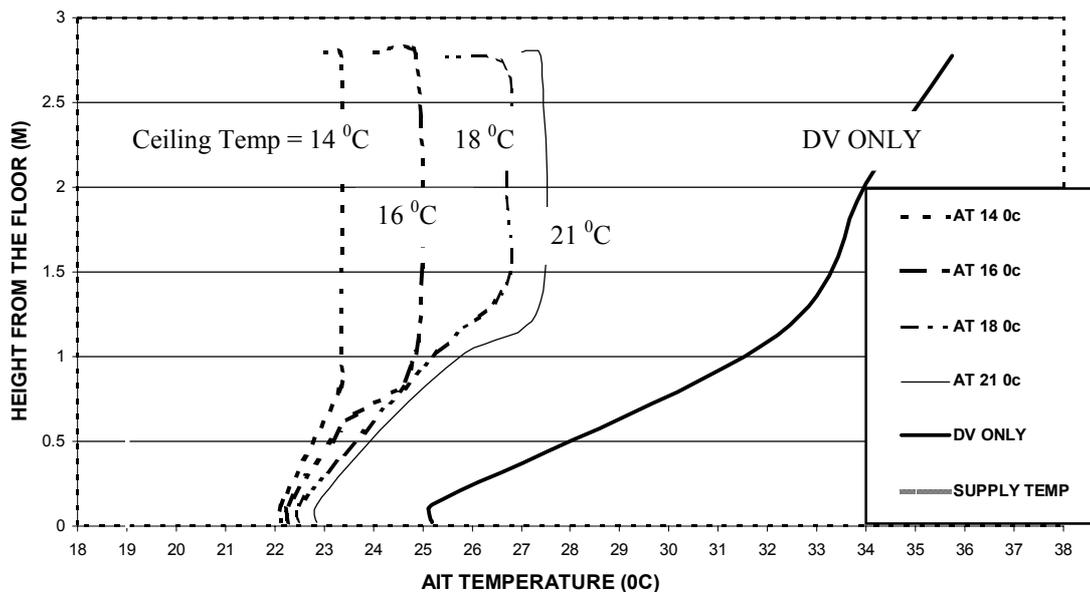
**Figure 2.** Air temperature versus height for a range of ceiling surface temperature at a heat load of 60W/m<sup>2</sup>.
