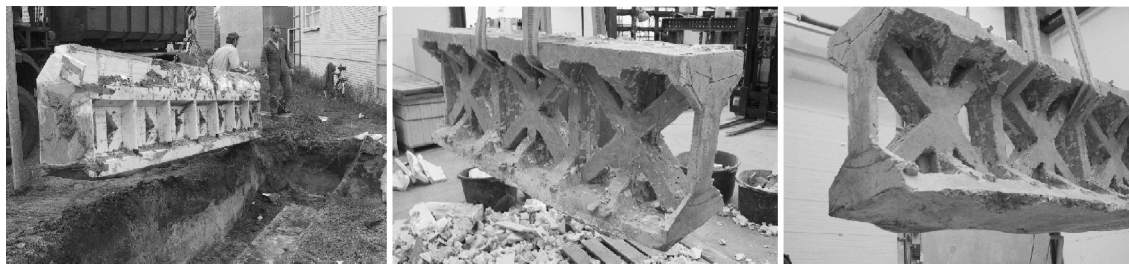
Figure 11: (Left:) the foundation beam is dismantled afterwards. (Middle:) and EPS-formwork is removed. (Right:) showing a completely filled beam with I-shape and truss structure.
