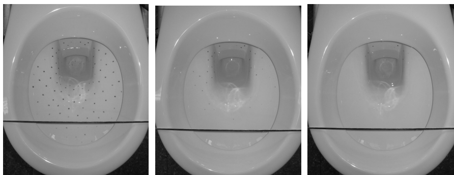
Figure 4 – Remaining dots after the first, second and third flushing
